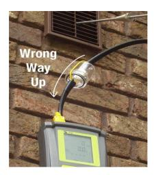
WARNING: - There is ONLY one correct way to connect the 'K' type thermocouple plug into the socket (see 2.4). The thermocouple plug is designed with one thick (negative) and one thinner (positive) prong. Forcing the plug into the socket the wrong way round may result in damage to the instrument. Failure to comply may result in damage to the instrument and will invalidate the warranty.
