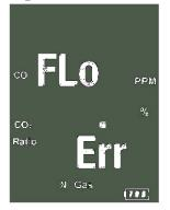
The 709R will also give off an audible Beeping Alarm to warn that a "FLo Err" is being detected
