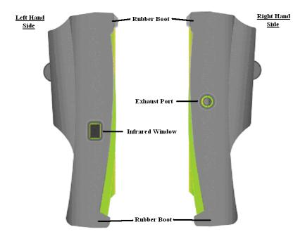
Exhaust Port Port for connection of Exhaust Adaptor
