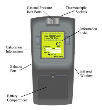
Gas and Pressure Inlet Ports Connection for In-Line Pump Protection Filter
