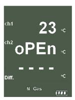
Displays Temperature reading of Channel 1 (ch1) in degrees Centigrade (°C) or degrees Fahrenheit (°F) Displays Temperature reading of Channel 2 (ch2) in degrees Centigrade (°C) or degrees Fahrenheit (°F) Displays the Differential Temperature (Diff.) between ch1 and ch2 in °C or °F
