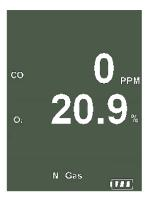
Displays Carbon Monoxide (CO) reading in parts per million (ppm)
