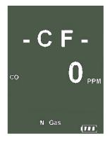
Displays CO air free calculated reading
