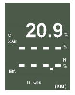
Displays Oxygen (O<sub>2</sub>) reading in percentage (%) Displays calculated Excess Air (X Air) figure in percentage (%)
