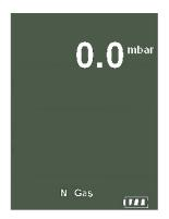
Displays Pressure reading in either millibars (mbar), kiloPascals (kPa), or inches of Water (inH<sub>2</sub>O)
